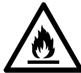
WARNING: Risk of fire
